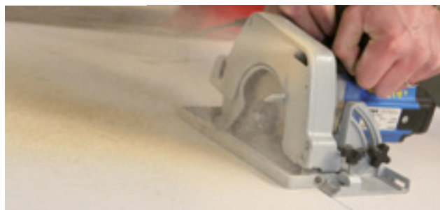
Picture No. 4: Cutting feed slower then for solid wood.
