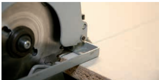
Picture No. 3: Cutting handheld circular saw.
