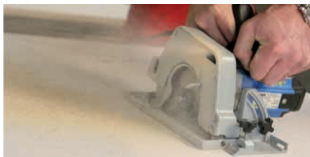
Picture No. 4: Cutting feed slower then for solid wood.
